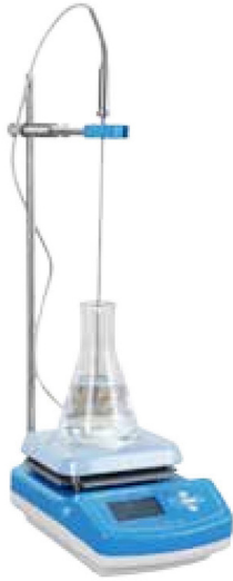
Magnetic stirrer to measure liquid temp.
